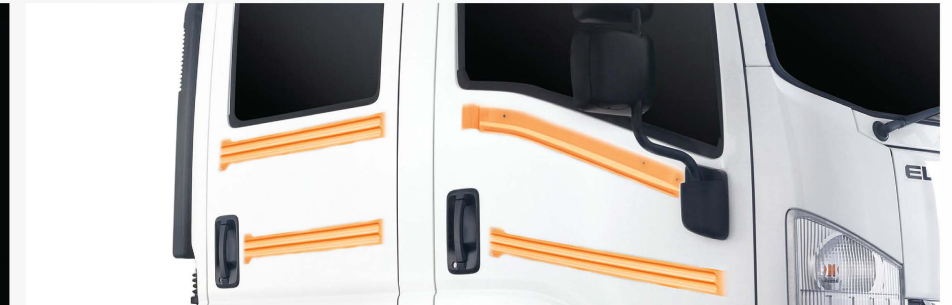
Door impact beam with high tensile strength reinforcement frame.
