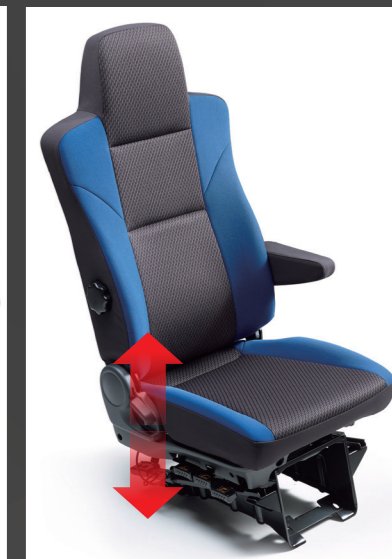
Air suspension driver's seat to provide maximum comfort.
