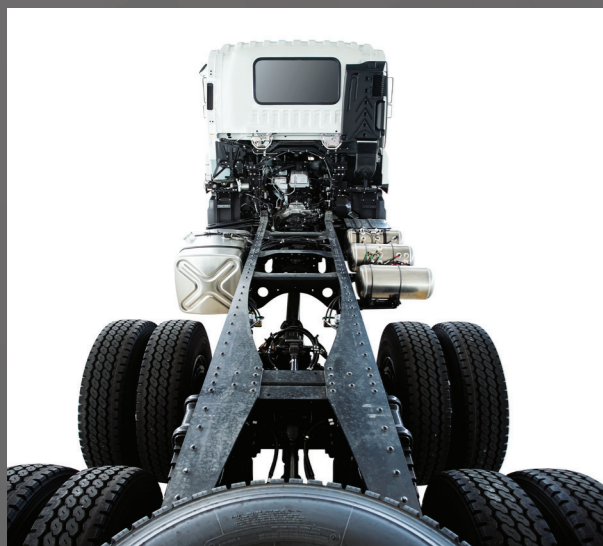
Double layer chassis frame.
