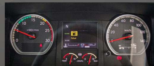
New multi information display meter with 4 inch LCD monitor.
